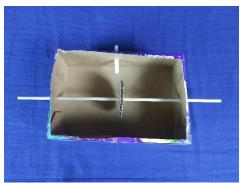
5. Slide half of a skewer in and glue a cam to the bottom. Add a cam to the top of that same skewer as shown.
