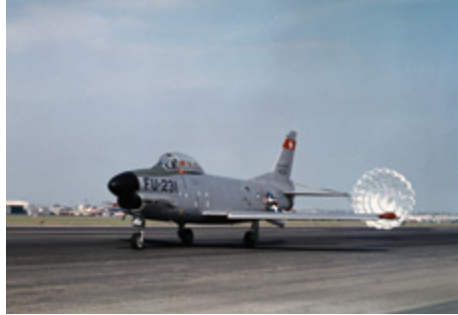
In the 1950s, this F-86 Sabre Jet used a drogue chute to help it land. © Boeing. All Rights Reserved.
