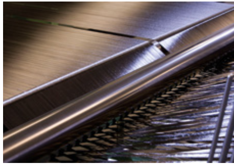
This is carbon fiber. It is used in the 787's fuselage and wings. © Boeing. All Rights Reserved.
